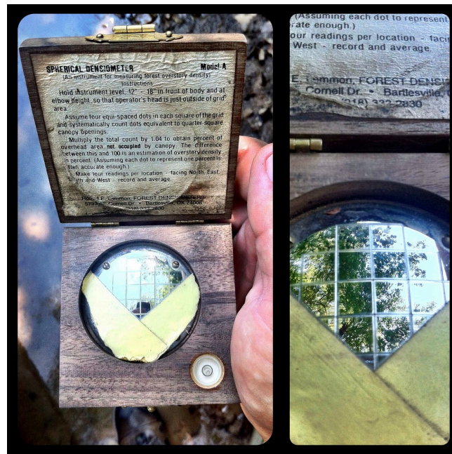
Figure 2. Example of how wedge-shaped area can be created with tape. Image from: www.flickr.com/photos/silentstcott/9895076415
